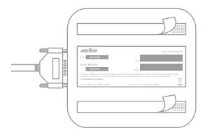
Motive recommends installing the Vehicle Gateway near the windshield, as well as away from any vents, electrical components and at least 12 inches away from any metal components.
