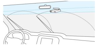
Top mounting location (recommended): Position the dashcam not more than 216 mm (8.5 inches) below the upper edge of the area swept by the windshield wipers. For most vehicles, the optimal location is to install on the right side just behind the rear view mirror.
