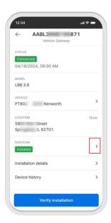
2. Test the mounting location 2.8 Make necessary adjustments to the Dashcam for clearer images if required. Tap refresh to display the updated images
