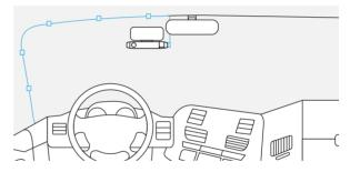
Use the provided cable clips to secure the dashcam cable around the edge of the windshield.
