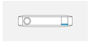
This should power up the AI Dashcam Plus and the right side LED on the AI Dashcam Plus should show solid blue after a few seconds of booting up.
