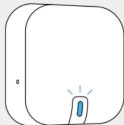
The LED will start blinking blue to indicate that the sensor is beginning the pairing process.
