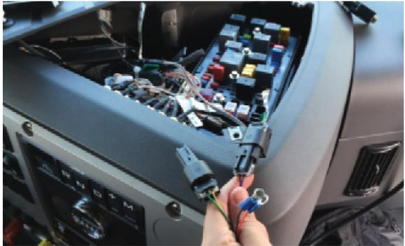
Several power/ground studs stick out of the truck inside the access panel. The Motive cable ring terminals fit over two of the studs, which should be labeled or color coded.
